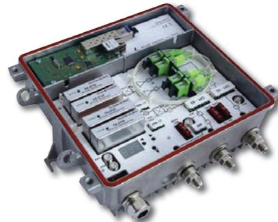
The ONS can be equipped with monitoring module including RJ45 or SFP interface.
